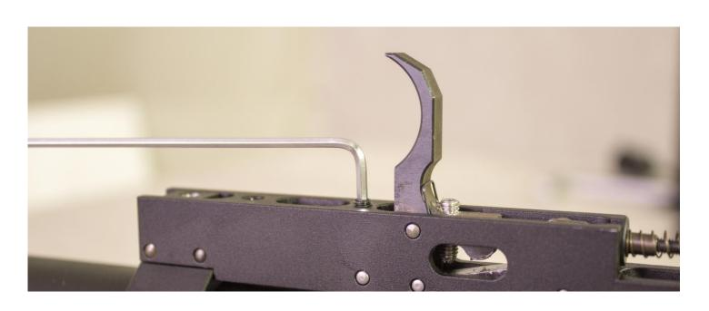
It is also possible to carry out this adjustment through the holes in the trigger guard without removing the bed.
