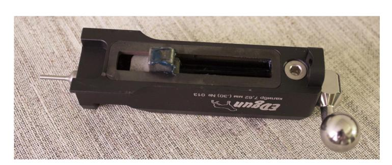
Note that the O-ring seal is located in the breech. Sometimes the the O-ring can fall out, sometimes it remains in the breech. Do not lose it. It the O-ring is missing you will feel a puff of air coming from the breech upon firing.
