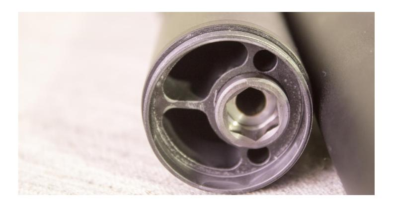
It is not recommended to completely disassemble the compression nut and clamping unit, as there is a possibility of losing fixing balls and springs.
